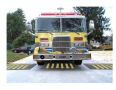
Speed cushions are a series of speed humps installed across the width of the roadway with spaces between them. The spaces are spaced so that emergency vehicles can pass between them without being affected by the bumps. Ordinary cars have smaller axels and will therefore need to travel over the bump with at least one side of their car. Speed cushions have about the same effect on slowing cars down as speed humps do while still allowing emergency vehicles to be unaffected by them.
