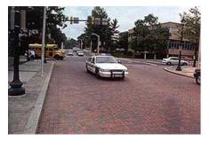
Textured pavement can be created by either stamping the pavement or by using an alternative material like brick or cobblestone. The purpose of both methods is to create a surface that is unpleasant to drive over at high speeds due to the uneven texture of the surface. If driven over at higher speeds the texture will cause a noticeable vibration to the car, much like a rumble strip does. The variation in the surface will also cause an audible difference when driven over. Generally the
